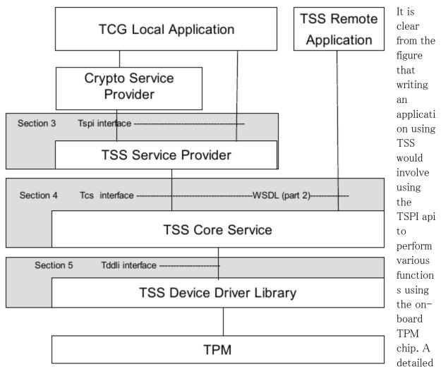
specification of the api can be obtained from the TSS specification. <a href="http://www.trustedcomputinggroup.org/resources/tcg\_software\_stack\_tss\_specification">http://www.trustedcomputinggroup.org/resources/tcg\_software\_stack\_tss\_specification</a>
